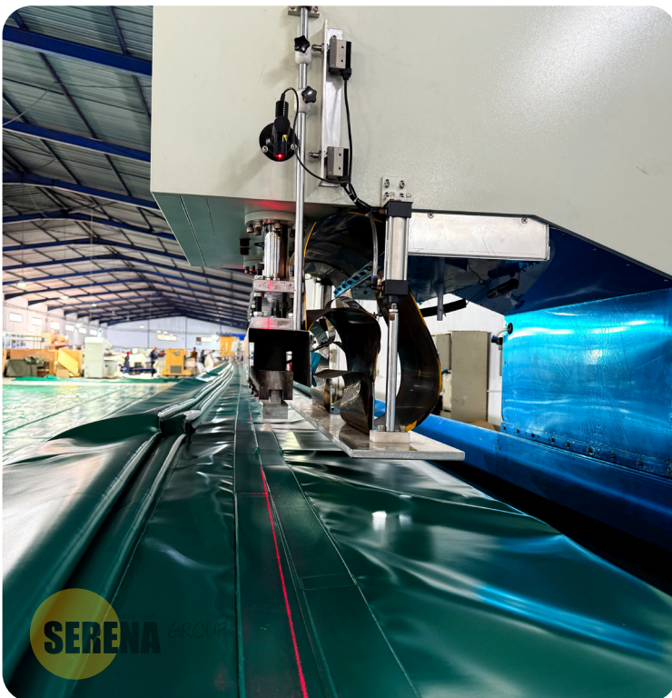
High Frequency welding machine on 30 metre long table
